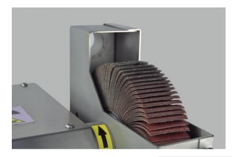
P7 incorporates one abrasive flap wheel of 200 mm diameter and 50 mm width.
