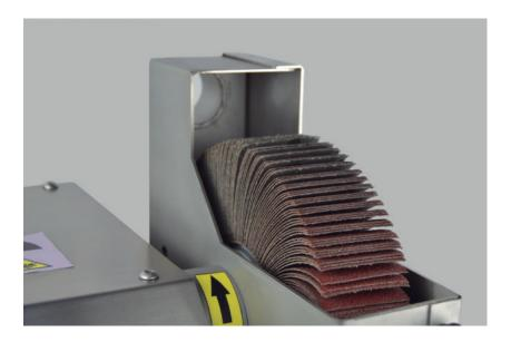
It incorporates one abrasive flap wheel of 250 mm diameter and 50 mm width, and 20 mm axis.
